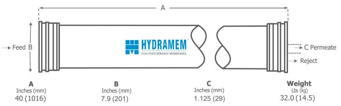
All Membrane Elements are supplied with a brine seal, interconnector and O rings
